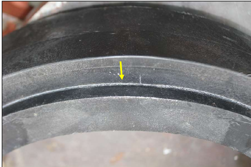
Figure 5: Photograph of Crack at Failure in Bottom of Riser
