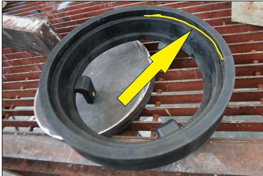
Figure 4: Photograph Showing Location of Crack at Failure on Top of Riser
